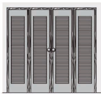
Double--folding louvered door: The ventilation area is 800 cm 2 ←
