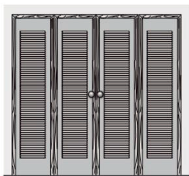
Double--folding-louvered door: The ventilation area is 800 cm²
