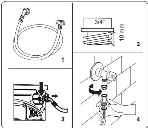
1. Your machine may have either a single water inlet connection (cold) or double water inlet connection (hot and cold) depending on the machine specifications. The white capped hose
