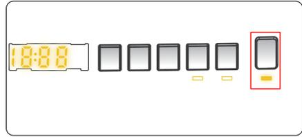
By pressing on the Start/Pause button, you may start the programme you have selected or suspend a running programme. If you switch your machine to the standby mode, the Start/Pause led on the electronic display will blink.
