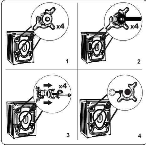
1. Before operating the washing machine, remove the 4 transit bolts and rubber spacers from the rear of the machine. If the bolts are not removed, they may cause heavy vibration, noise and malfunction of the machine and void the warranty.
