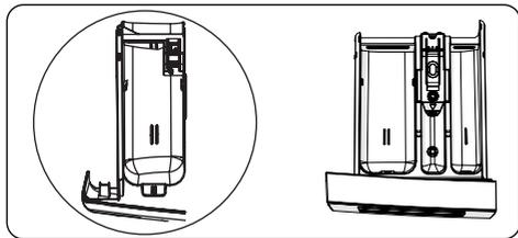
This compartment is for liquid or powder detergents or limescale remover. The fluid detergent level plate will be supplied inside your machine. (\*)
