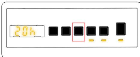
You can use this auxiliary function to delay the start time of the washing cycle for 1 to 23 hours .
