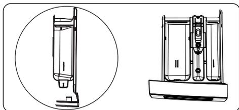
This compartment should be used only when the pre-wash feature is selected. We recommend that the pre-wash feature is used only for very dirty laundry.
