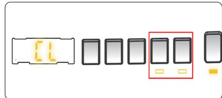
If any button is pressed or selected programme is changed by the programme dial while the child lock is active, the "CL" symbol will flash on the electronic display for 2 seconds.
